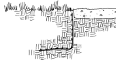
Figure 9. Various ways to install a barrier to prevent coyotes from digging under chicken coops and similar places. To add to the life of the barrier, spray on two coats of rustproof paint before installation. Always check for utility lines before digging in an area. (Drawings by Jenifer Rees.)
