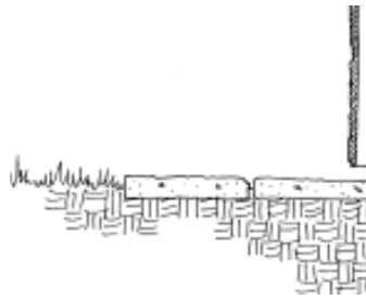
Figure 9. Various ways to install a barrier to prevent coyotes from digging under chicken coops and similar places. To add to the life of the barrier, spray on two coats of rustproof paint before installation. Always check for utility lines before digging in an area. (Drawings by Jenifer Rees.)
